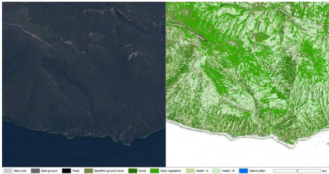
Figure A2.15: Comparison of raw satellite imagery with the output from the Maximum Likelihood Classification on the GeoEye-1 data – section G
