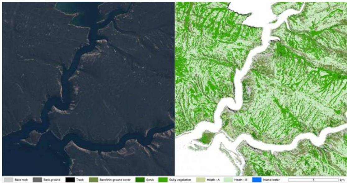
Figure A2.16: Comparison of raw satellite imagery with the output from the Maximum Likelihood Classification on the GeoEye-1 data – section H
