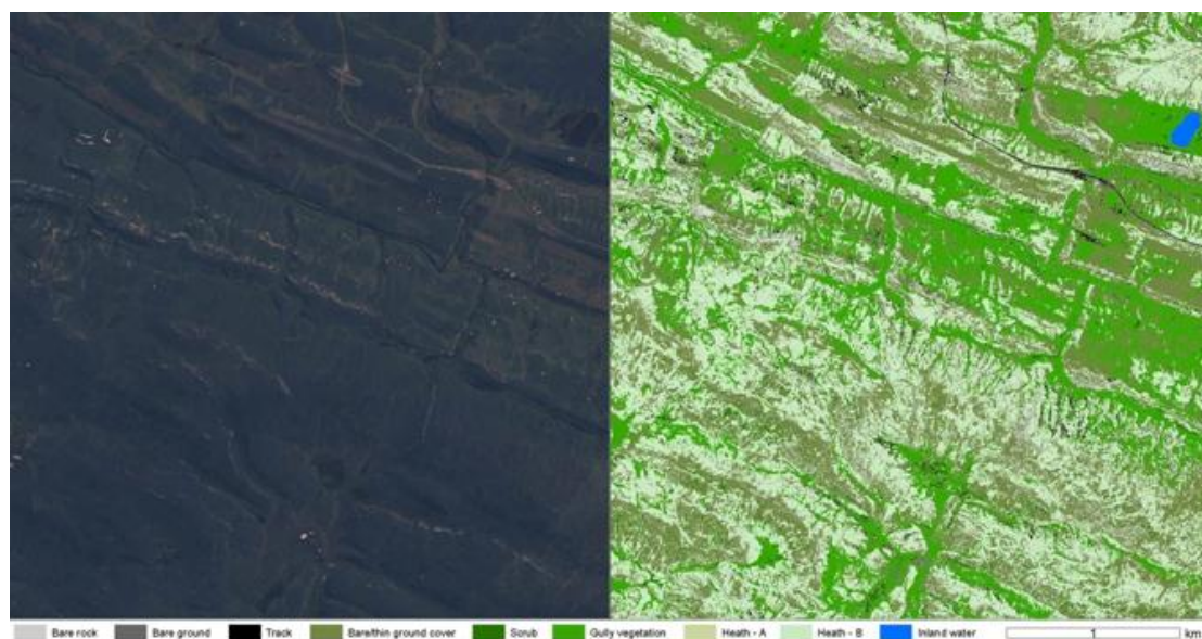
Figure A2.13: Comparison of raw satellite imagery with the output from the Maximum Likelihood Classification on the GeoEye-1 data – section E
