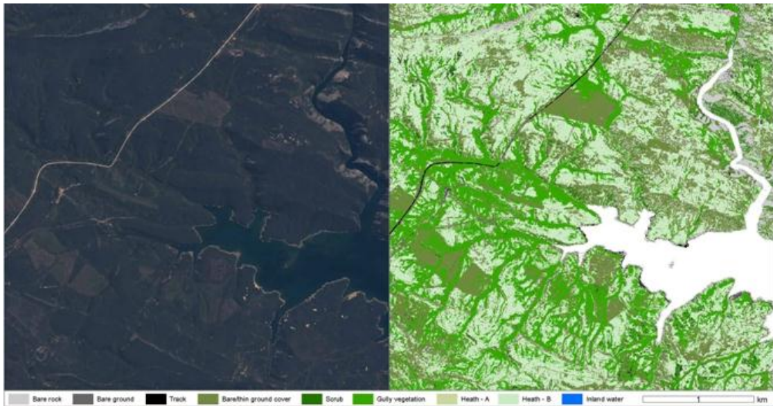
Figure A2.11: Comparison of raw satellite imagery with the output from the Maximum Likelihood Classification on the GeoEye-1 data – section C
